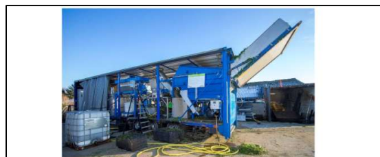
GBR Grassa Location: mobile concept, the Netherlands Founded: 2014 Feedstock: fresh grass or green feedstock (e.g. tomato stems, waterplants) Capacity: 300 – 600 kg per hour Investment costs: ca. 600,000 Euro Runtime: 5 months of year (3,000 hours, diversification of feedstocks to lengthen season)
