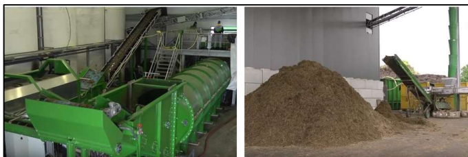
GBR NewFoss Location: Uden, the Netherlands Founded: 2016 Feedstock: silage grass (grass is provided by Staatsbosbeheer) Capacity: 10,000 t dm /a (40,000 t grass per year) Investment costs: n.a.
